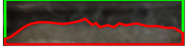
(b) Obtained fractional area of the morphologies (red enclosures) for \mathbf{D} = 0.8 (top) and \mathbf{D} = 0.4 (bottom) used for computing dendrite measure \bar{\lambda} .
