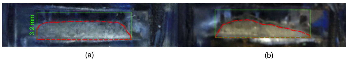
FIG. 2. Naked-eye observation of in situ lithium dendrites created at i = 2 \text{ mA cm}^{-2} for t = 24 \text{ h} (a) before and (b) after submerging in the oil bath of T = 78 \text{ }^\circ\text{C} for t = 48 \text{ h} . The filled area fraction has been reduced from 64% to 41%.
