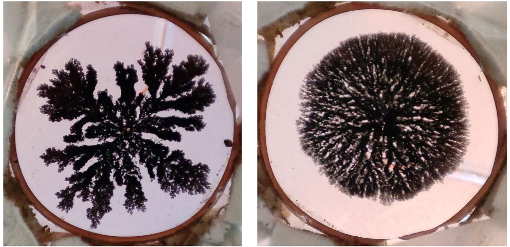
(a) Branched morphology formation for (C_0, V_0) = (10mM, 3V) at t = 500s . (b) Packed morphology formation for (C_0, V_0) = (10mM, 5V) at t = 180s .
