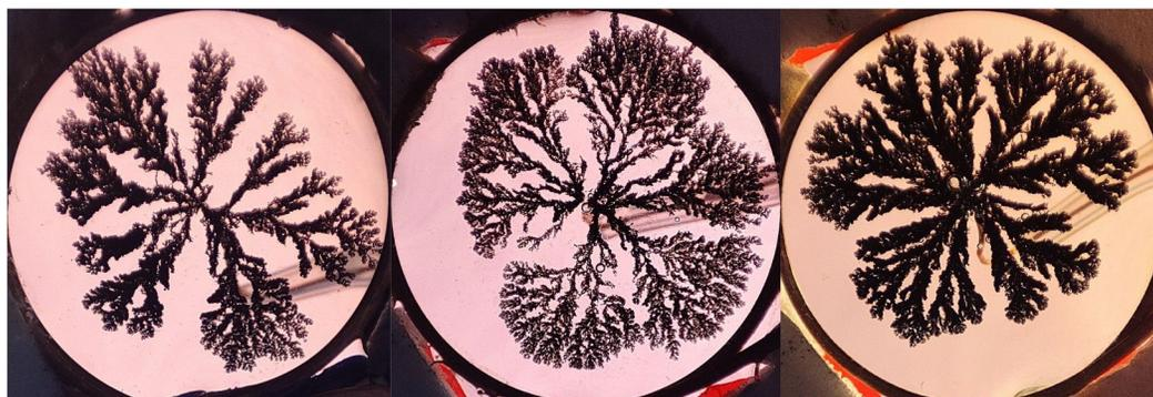
(a) Branched morphology samples formed at  $\{C_0, V_0\} = \{(5, 5, 10) \text{mM}, (4, 5, 5) \text{V}\}$  and times  $t = \{440, 360, 200\} \text{s}$  respectively.
