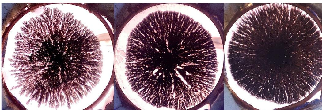
(b) Packed morphology samples formed at  $\{C_0, V_0\} = \{(10, 25, 25) \text{mM}, (6, 6, 6) \text{V}\}$  and times  $t = \{150, 120, 150\} \text{s}$  respectively.
